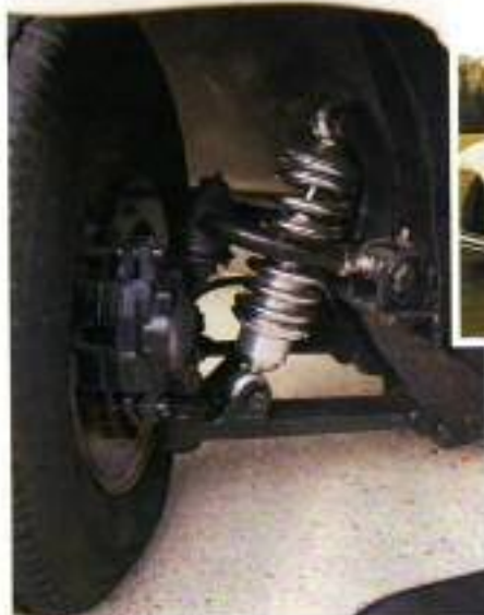
Dirt track-bred Martz front suspension combines tubular A-arms and PRO Shocks coilovers.
