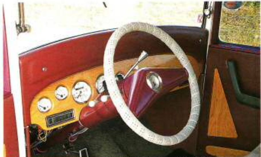
Diminutive oak dashboard snugly accommodates air conditioning outlets. Steering column is GM.
