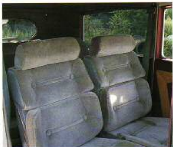
Nissan Maxima front seats are a perfect fit in the Plymouth's narrow interior.
