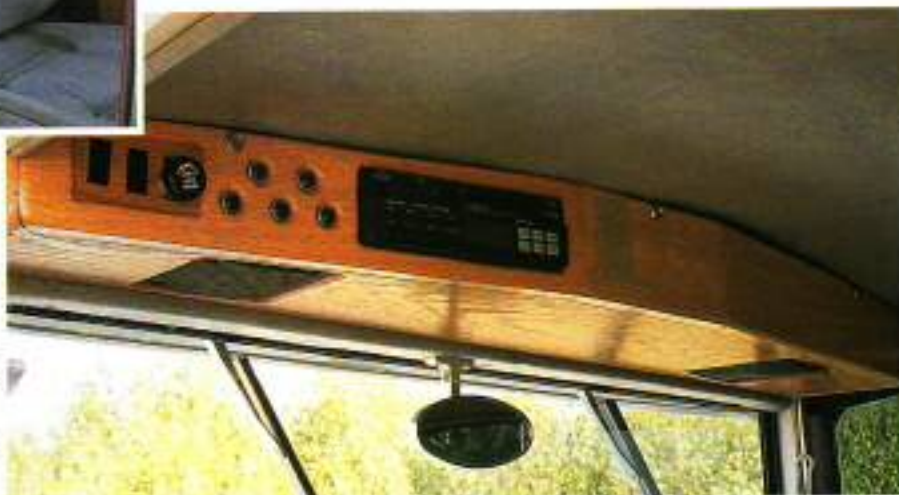
Audio components and controls fit neatly into home-built oak console above windshield.
