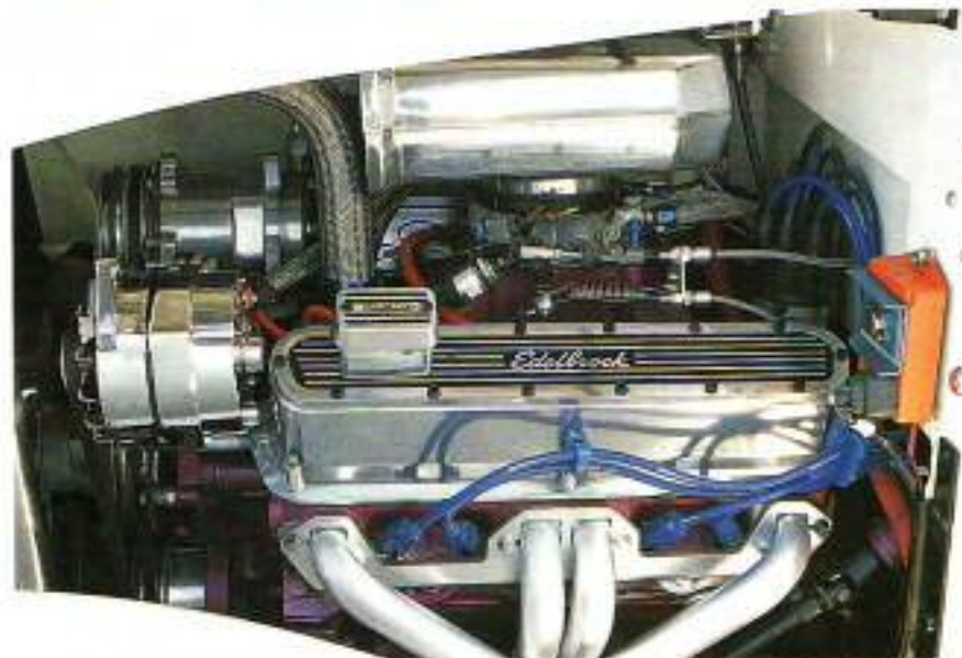
340-cu.in. Plymouth engine has a Holley throttle-body fuel injection, ported heads and Sanderson headers.
